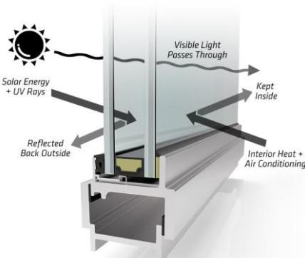
Bi-Fold systems come with energy-conserving glass that lets the light through, but keeps the warmth inside and the cold outside.
